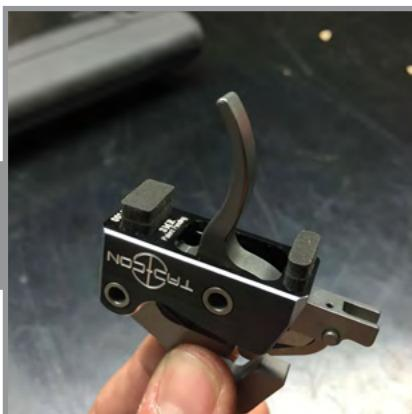
If installation of additional pads is necessary, use a small amount of adhesive to secure each pad to the corresponding pad, stacking them as shown in photo
